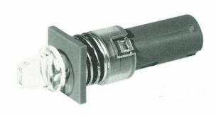
This model is not a switch since it has no contacts. The position indicator is simply a dummy and just aids the operator by the optical indication of a positive switching or working condition. It is turned manually to the required position in accordance with observation of a conditional change, or on a remote signal, without initiating any further function.
